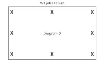
X = Location of orange pan head screws attaching the sign to the plywood. Set screws as indicated, keeping screws 2" inside the sign's outside border.
